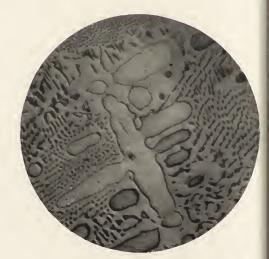
Fig. 18. Type of Class 2. Iron containing 8 per cent. P. Magnified 250 diameters.
